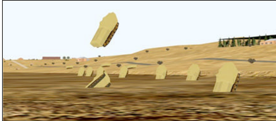
A visualization of SAF vehicle behaviors after encountering topological construction featuring “T” vertices along adjacent polygons
